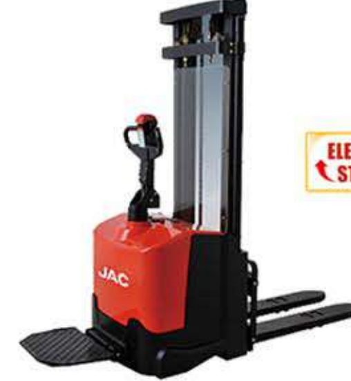
Model: CDD12-II / CDD14-II / CDD16-II / CDD20-II Load: capacity: 1200kg / 1400kg / 1600kg / 2000kg Standard lift height: 2000-4000mm Overall fork width: 550-685mm Fork length: 1150mm Battery voltage/capacity: 24V/280Ah
