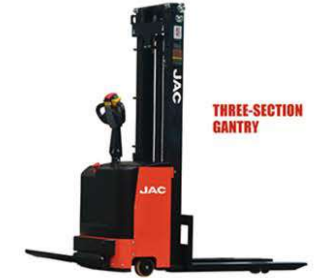
Model: CDD20-I / CDD20-I Three-section gantry Load: capacity: 2000kg / 2000kg Standard lift height: 1600-4000mm / 4000-5000mm Overall fork width: 570/695mm Fork length: 1150mm Battery voltage/capacity: 24V/210Ah / 24V/280Ah
