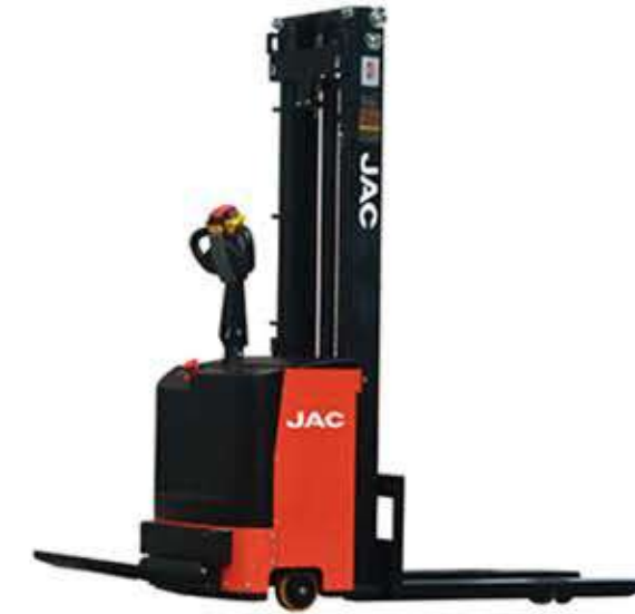
Model: CDD10-I / CDD12-I / CDD15-I Load: capacity: 1000kg / 1200kg / 1500kg Standard lift height: 1600-4000mm Overall fork width: 570/695mm Fork length: 1150mm Battery voltage/capacity: 24V/210Ah
