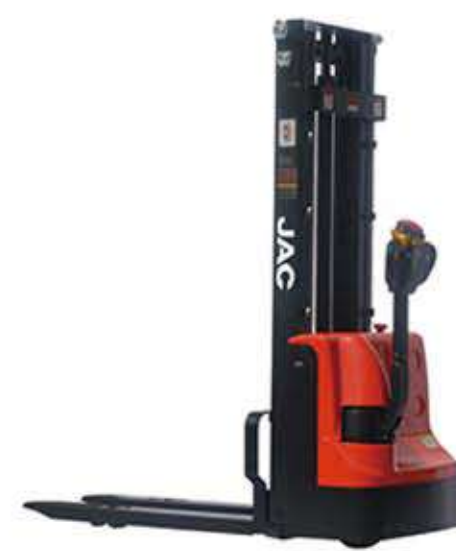
Model: CDD10-I / CDD15-I Load: capacity: 1000kg / 1500kg Standard lift height: 1600-3500mm / 1600-3500mm Overall fork width: 570/695mm Fork length: 1150mm Battery voltage/capacity: 2x12V/100Ah
