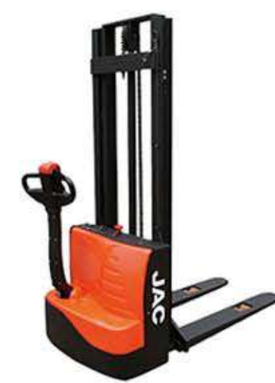
Model: CDD10-II Load: capacity: 1000kg Standard lift height: 2000-3300mm Overall fork width: 550/685mm Fork length: 1150mm Battery voltage/capacity: 2x12V/70Ah
