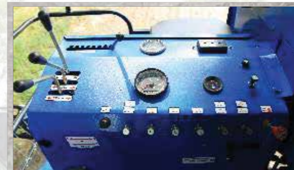
3 forward and 1 reverse gear which makes combine more efficient
