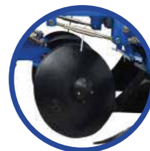
SHOVEL AND DISC MADE OF BORON STEEL
