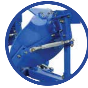
FURROW ANGLE ADJUSTMENT FOR BIGGER FURROWS
