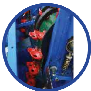
QUICK UNLOCK OPTION TO CHANGE PLANTING BELTS
