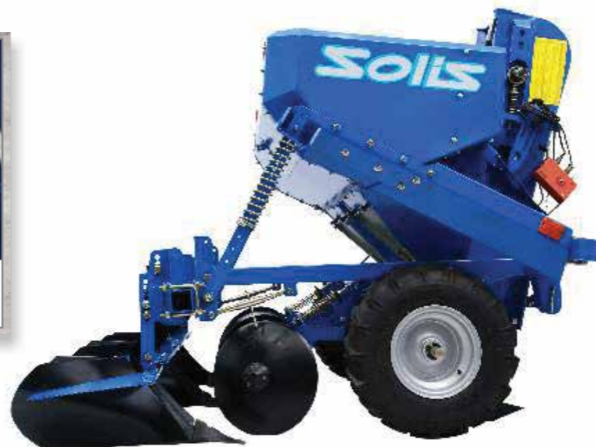
Furrow opener with replaceable wear and tear point and depth adjustable spike
