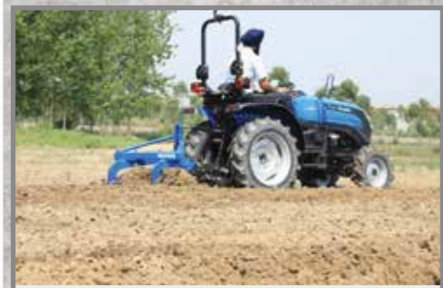
Specially designed for breaking, raising turning & mixing of soil.
