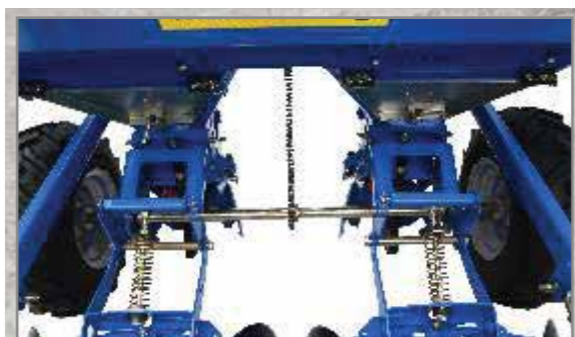
Heavy duty height adjustable axle
