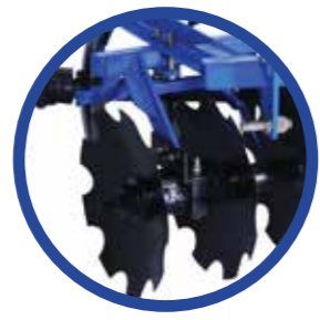
USED FOR CHOPPING UP UNWANTED WEEDS OR CROP RESIDUE
