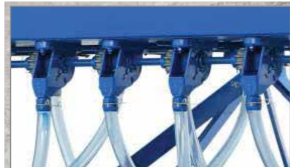
Seed sowing with help of precise seed metering system
