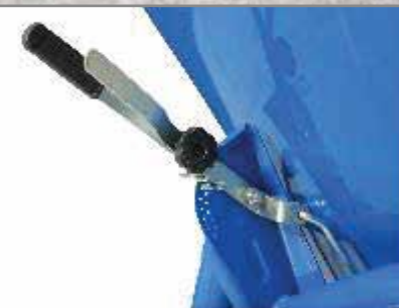
Provision of spreading direction lever which enables better spreading of fertiliser
