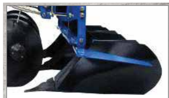
Rigid and concave shaped mould board for proper ridge formation
