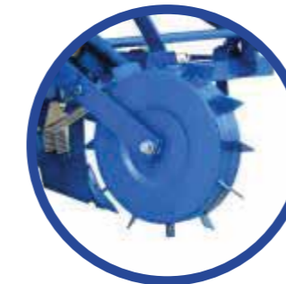
ADJUSTABLE DEPTH CONTROL WHEELS
