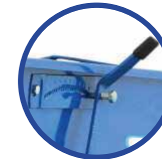
SIMPLE LEVER TO ADJUST SEED AND FERTILISER RATE
